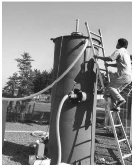
Fig. 5 Orifice flow meter of Kamisu-Wakamatsu hot spring source.
